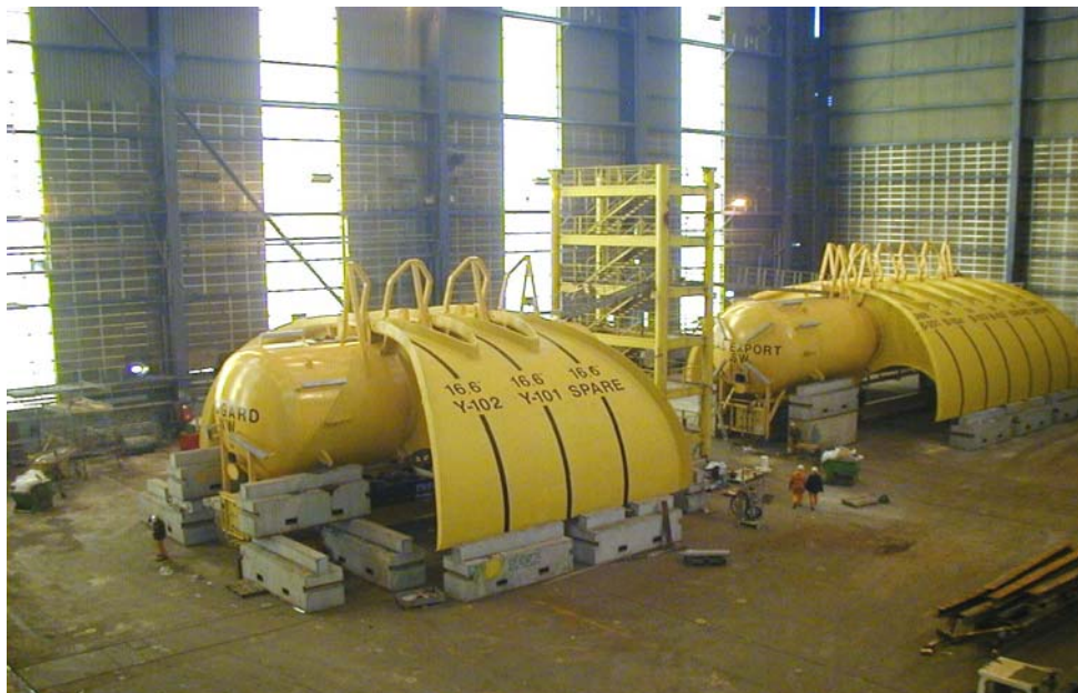
Trays designed by FiReCo to support risers from sub sea wellheads to surface
